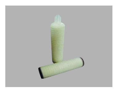
amcAccuFlow cartridge is a precision filter product that combines the benefit of both a prefilter and final filter in one device to provide reliable and consistent performance. The pleated filter medium is amcAccupor membrane, i.e., modified hydrophilic polyethersulfone membrane specifically developed by AMC for various filtration applications.
